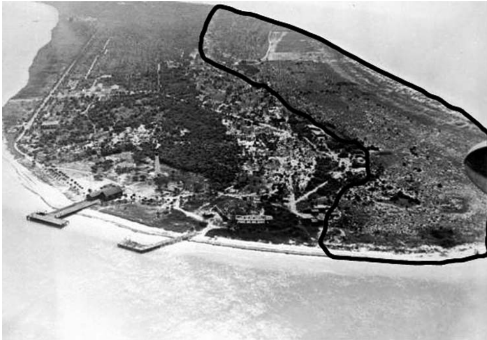
FIG. 1. Aerial view of the northern section of Egmont Key in an undated photo probably taken in the early to mid-1900s. The area outlined in black has completely washed away; it amounts to nearly one-half of the island that was present in 1875. Photo from the Florida State Archives (Number N046232), Tallahassee, Florida, USA.
